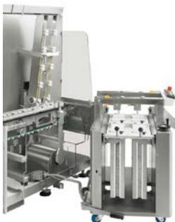
At site level, Mediseal's LSC® "Late Stage Customization" concept enables manufacturers to cleverly combine small batches of packaging and assemble them later. Standardized, unprinted or partly printed blisters are collected in BIB-BOB modules and later printed and cartoned together for specific customers.
