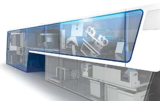
*Mediseal BE Blister Series: The circulating blue line maps the flow of product through the machine and as it narrows it symbolizes the merging of the product. In the event of faults, it serves as an illuminated display element to provide rapid assistance to the operator.*
