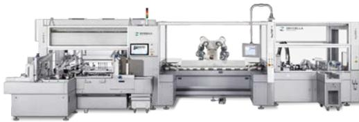
*Dividella NeoTOP x – highly flexible TopLoad packaging machine for processing small to medium lot sizes, equipped with a collaborative robot for the greatest possible filling flexibility.*
