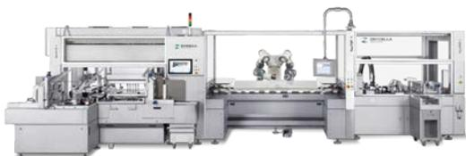
*Dividella NeoTOP x – highly flexible TopLoad packaging machine for processing small to medium lot sizes, equipped with a collaborative robot for the greatest possible filling flexibility.*
