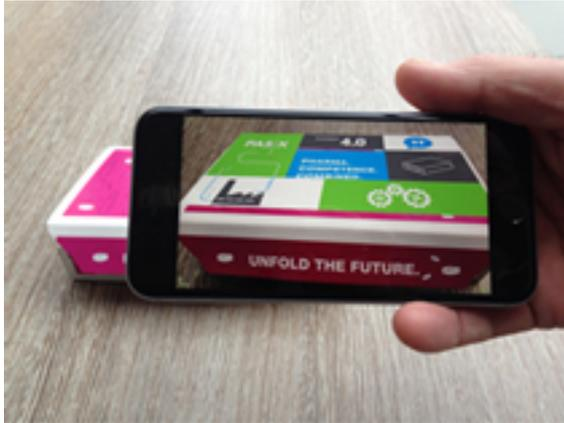
*The Rondo app reads reference points on the pack which are invisible to the naked eye and generates an Augmented Reality on the smartphone.*
