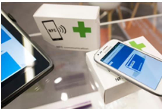
*The NFC chip is incorporated when the packaging is manufactured and transmits its information by radio as soon as a terminal which can read it is within range.*
