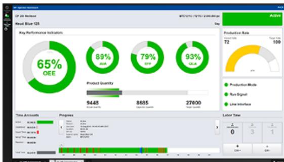
*PAS-X KPI for real-time monitoring of production and packaging installations*
